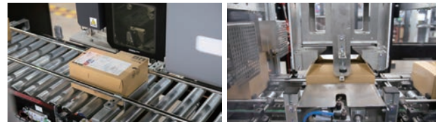
I-Pack® (high-speed automated packaging and shipping line) is capable of packaging and preparing a maximum of 720 packages for shipping in just an hour
