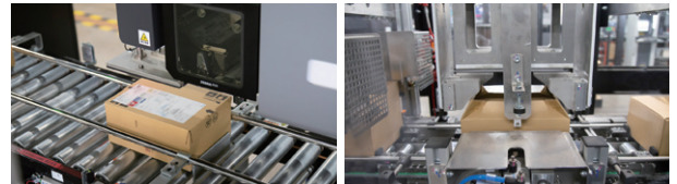
I-Pack® with a maximum packaging capacity of 720 pieces/line per hour (high-speed automated packaging and shipping line)
