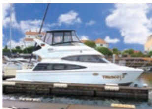
TRUSCO'S II (Ashiya) Length: Approx. 36.00 ft. (10.98 m) Weight: Approx. 12 tons, Capacity: 12 persons Horsepower: 285 (3,600 cc) × two engines
