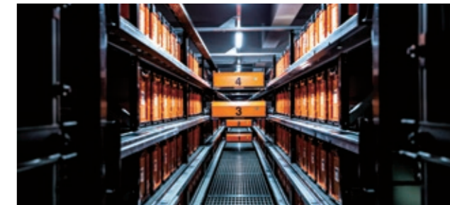
SAS (Systema Streamer) for “NIAWASE” (Order Consolidation) – bundling together multiple orders [high-speed load assorting equipment]
