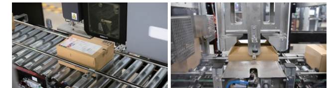
I-Pack® (high-speed automated packaging and shipping line) is capable of packaging and preparing a maximum of 720 packages for shipping in just an hour
