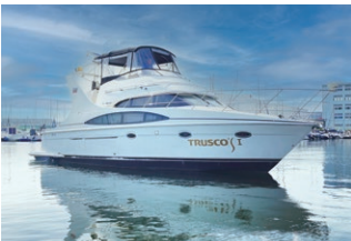
TRUSCO'S I (Yokohama) Length: Approx. 41.00 ft. (12.50 m) Weight: Approx. 18 tons, Capacity: 12 persons Horsepower: 370 (5,460 cc) x two engines
